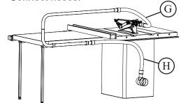
Contractor saw: make sure hose clears motor as the blade moves through its full range of elevation and tilt.
