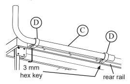
3. Tighten the screws that clamp tube C.
