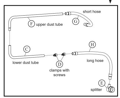
1. Slide clamps D onto tube C.
